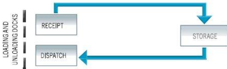
Simple Flow: Goods received, stored, and dispatched in the same unit load format. Source: Mecalux Technical Warehouse Manual
